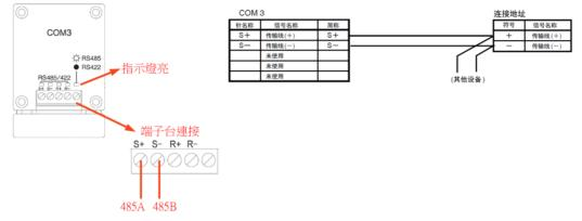
III. Connect AFPX-COM3's terminals (S+ ` S-) to the interface module (Pin1 and Pin2). The interface module is connected to the control module via the Ethernet cable connected to its RJ45 port
